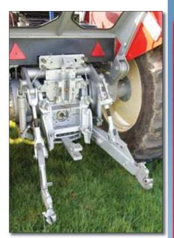
Above: The rear lift has a capacity of six tonnes and is fitted with a category III linkage. Michael believes his tractor previously pulled a five-furrow Ransomes
